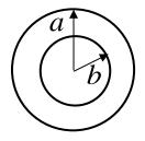
The cross-sectional area of the annulus shown is  $\pi(a^2 - b^2)$ , while the wetted perimeter is  $2\pi(a+b)$ . Therefore, the equivalent diameter is obtained as
