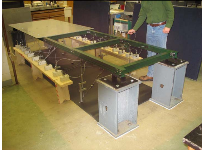
Figure 1: Laboratory Bridge Model for Diagnostics and Damage Detection
